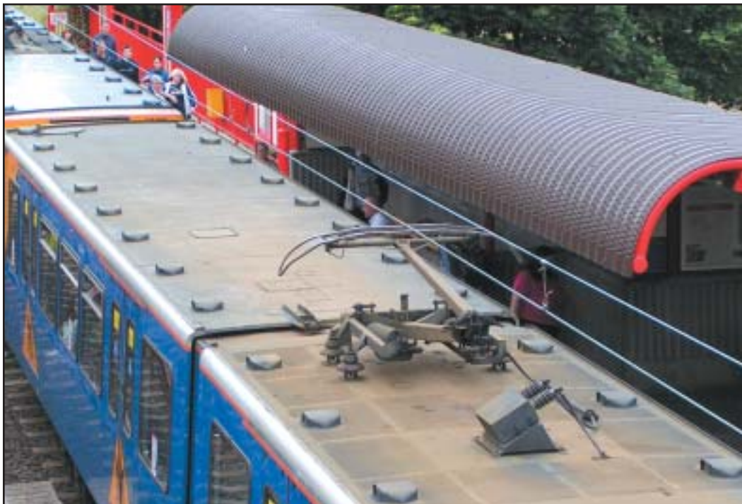
Metro's overhead wires carry 1,500 volts of electricity in the wires
